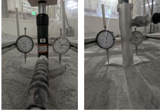
Figure 2: Plate, ram, and dial gauge conditions of standard 6" plate (left) and TRIDENT footpad (right).
